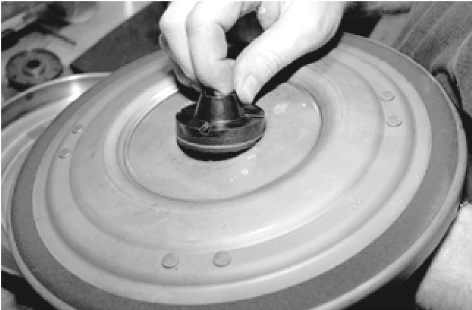
*This phenolic insert sets end-play and seals the input shaft to the clutch hub as well as determines overall converter height. They come in various sizes for adjustments.*
