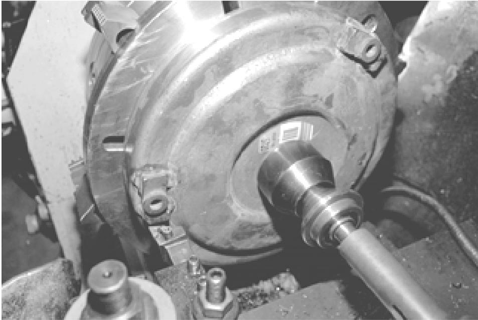
*The front half is flipped over and the mounting lugs are trued. You'd be surprised to find how many of these are crooked, beat up, or stripped.*
