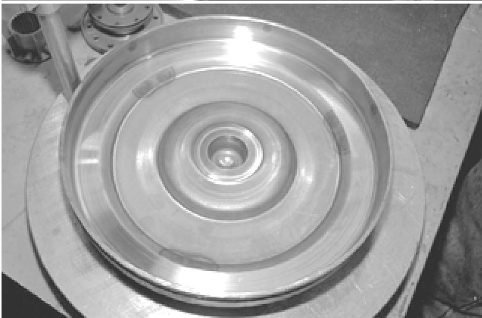
*The clutch rides on the front half of the converter cover. The contact area must be smooth, clean, flat, not burned, and not grooved or it gets chucked out. There is no effective and economical repair for damaged parts.*
