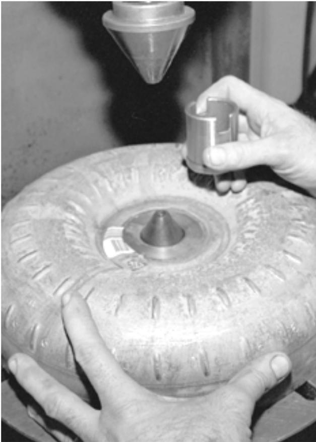
*The new hardened hub sets on the converter housing in a special jig. The housing rests flat and the conical fitting locates the hub in the dead center.*
