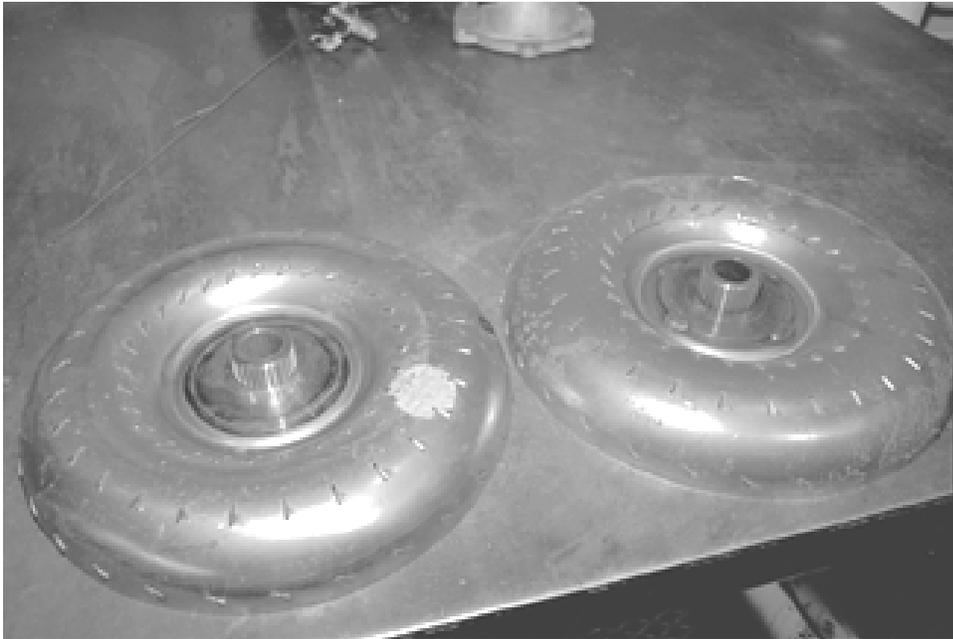
*The turbine on the right is an early multi-part unit with spot-welded hub. The one on the left is the late-style one-piece with full-perimeter welded hub that is the preferred part.*
