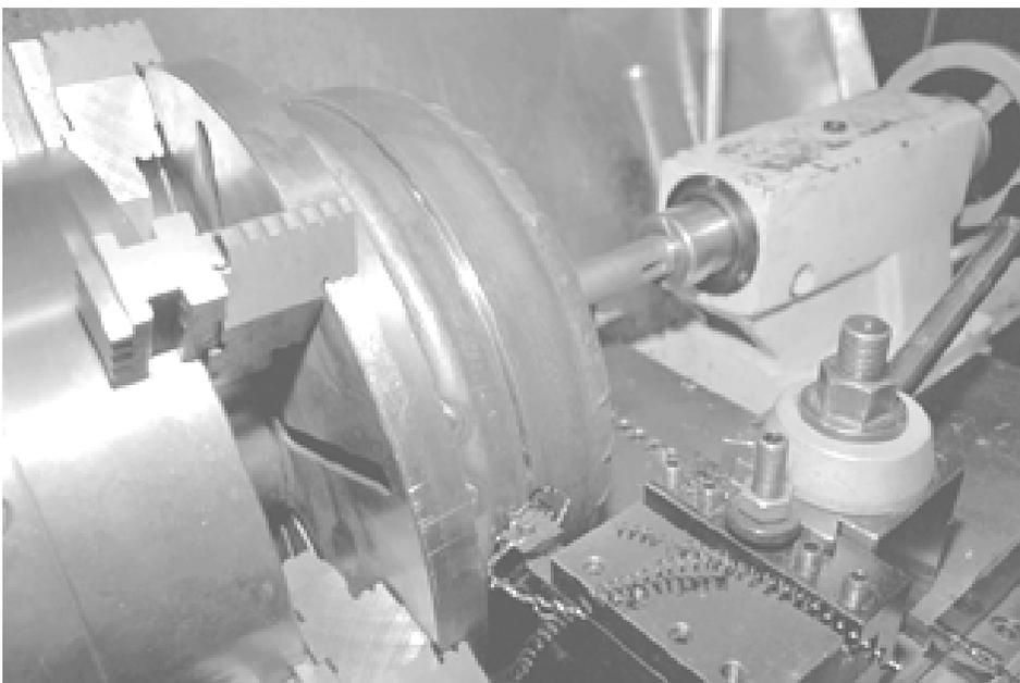
*The converter is cut apart in a lathe which cuts away the weld holding the halves together.*
