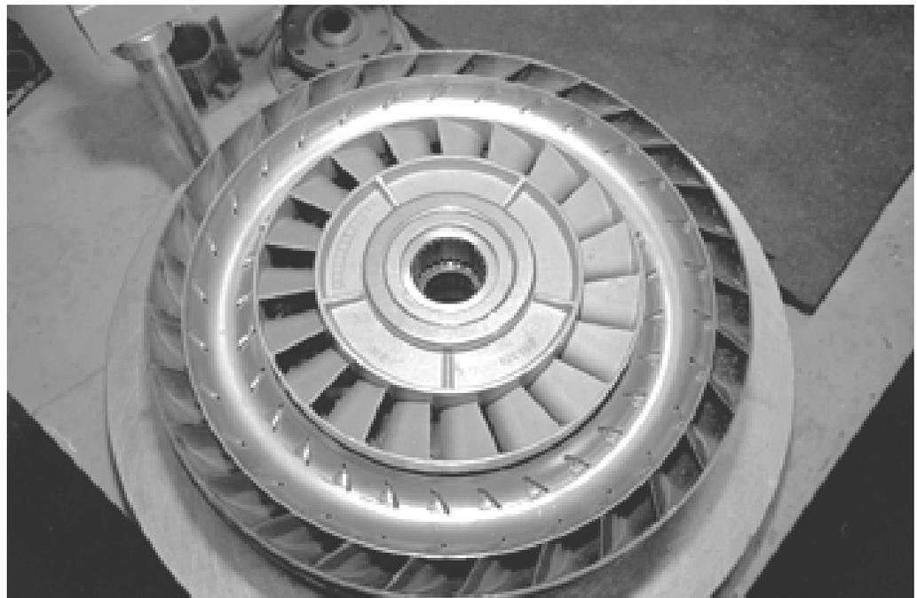
*The height and run-out are checked I the welding machine/jig before any welds are made. Alignment is critical and can make or break a converter.*
