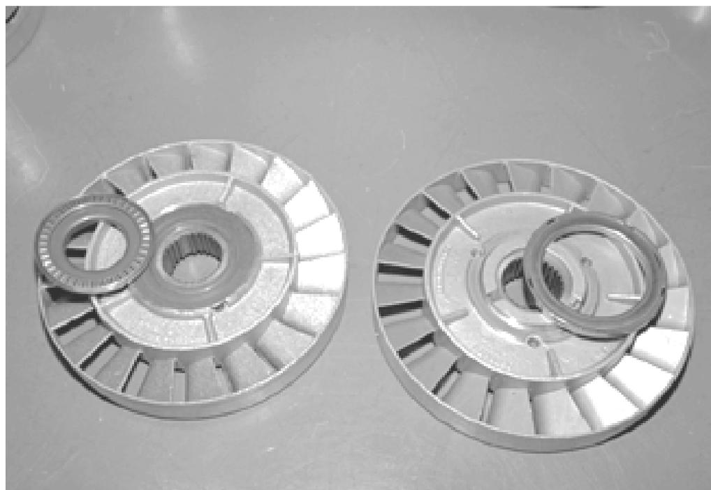
*The stator on the right is the late-style part with the large one-piece enclosed Torrington bearing. The other is the early style with the small Torrington with separate staked-in race. The right choice is obvious.*
