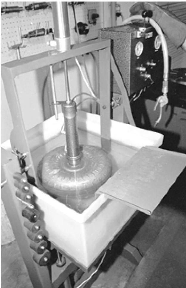
*All converters are pressure-tested at 120 psi. Not even the smallest leak is acceptable.*
