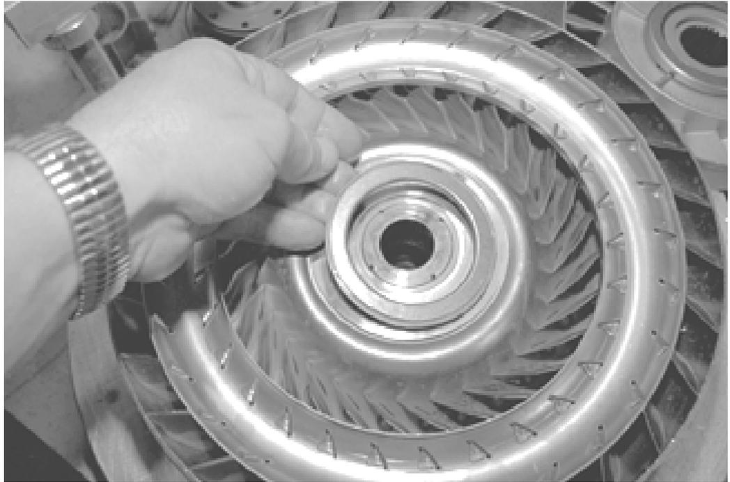
Speaking of conversions, there is a special hub made to replace the entire lock-up clutch assembly to eliminate lock-up. This is sometimes used in off-road or very high performance units where the clutch is either not needed or has the potential to cycle too often or even outright fail due to extreme abuse. In almost every case, a street vehicle performs best with a properly functioning locking converter.
