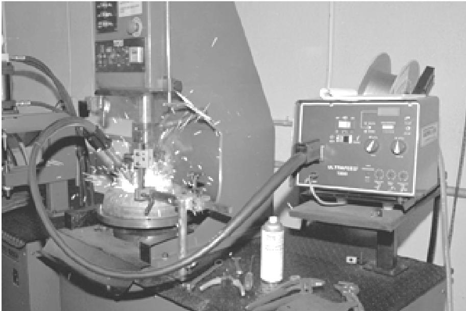
*The entire jig is part of a welding rig. The turntable rotates and a perfect, consistent weld is made around the hub. This robot welding is far better than can be hand-done.*
