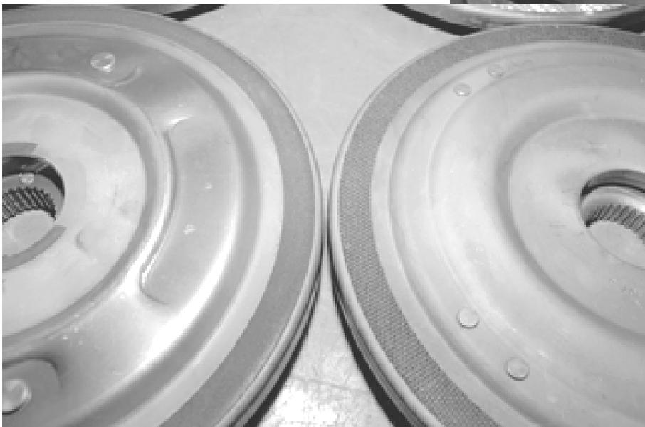
*On the right is the woven carbon fiber clutch used in 1998 and later severe duty units. On the left is the carbon composite clutch which is a durable and heat-resistant material used in most applications 1992-98.*
