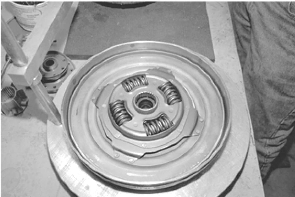
*The late HD clutch damper with the Kevlar clutch face seat in the front half of the converter housing.*
