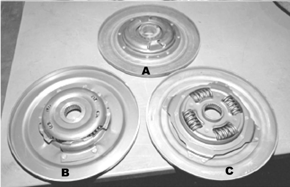
The common clutch damper units. (A) is the early HD damper, (B) is the late HD and performance damper, and (C) is the standard car and light truck unit.
