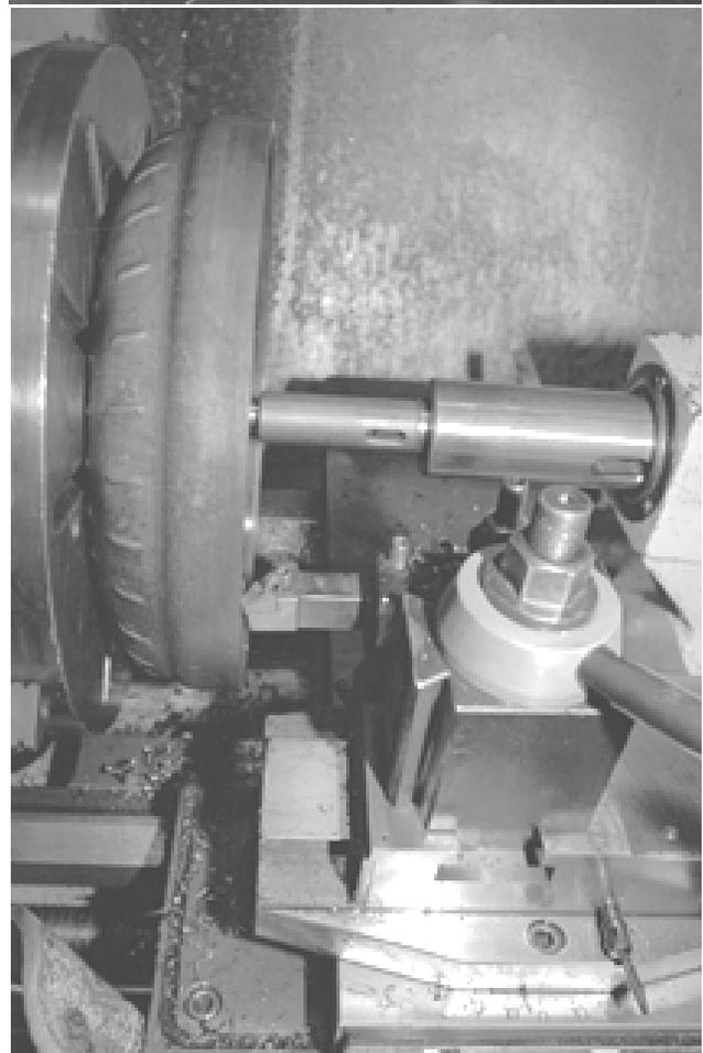
*The front half is also turned to clean weld debris and deepen the shelf cut so the halves can be assembled at the correct height later.*
