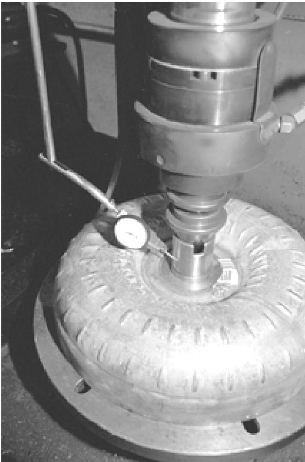
*Minute adjustments are done according to a dial indicator. The hub must be indicated to have no more than .001 inch of run-out.*
