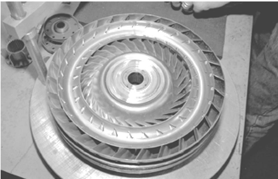
*The modified and silicon-bronze welded turbine is next in line over the clutch.*
