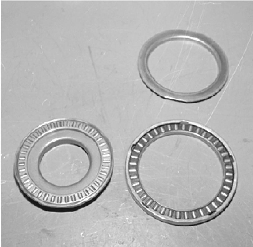
*The large bearing (opened up for the picture) not only has more bearing rollers but more contact area to spread the contact energy across. Less friction and less heat buildup.*
