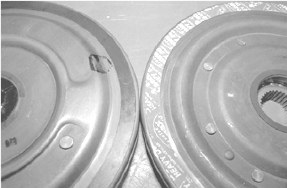
On the left is a paper faced clutch which is only good for the lightest-duty applications and which Phoenix never uses in its converters. On the right is the Kevlar material Greg bonds to upgrade or replace worn facings.
