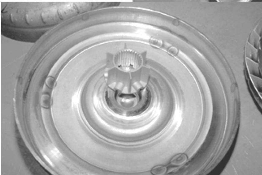
*If you want to eliminate the lock-up, the entire clutch assembly can be replaced with this machined hub/spacer.*
