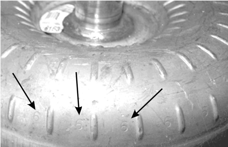
*The stamped numbers in many converters tell you details about stall speed and impellers. See sidebar #1*
