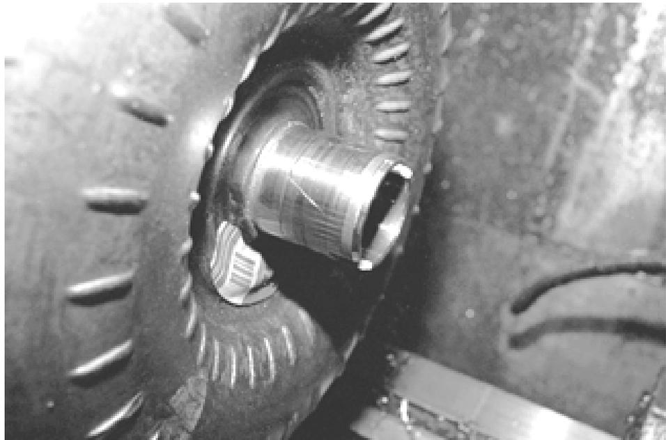
*The hub mount surface must be turned flat and smooth or it could end up defective.*
