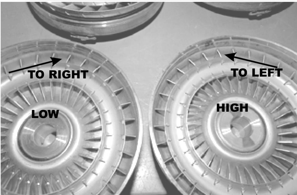
Blade angle is the way stall speed is determined. The low stall impeller fins angle to the right for less aggressive fluid movement. The high stall unit on the right has blades angled to the left which really increases fluid pressure against the stator.
