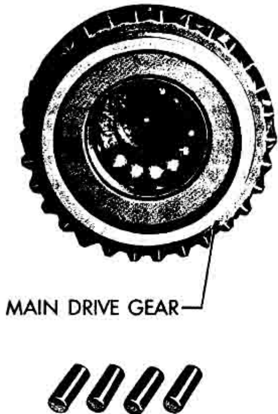
Fig. 20 Installing Bearing Rollers
