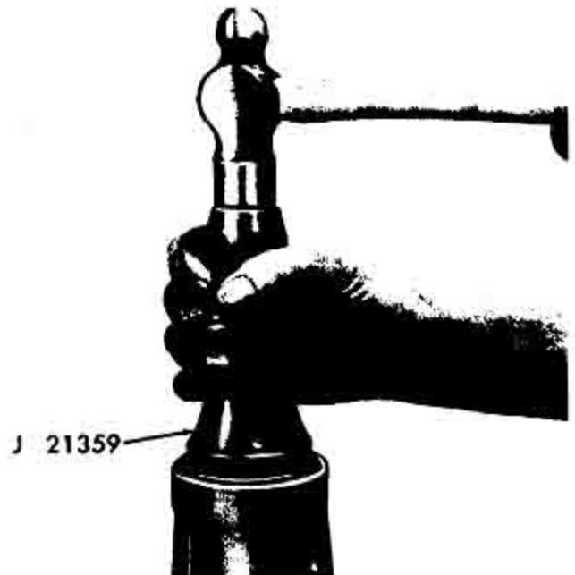
Fig. 14 Installing Case Extension Oil Seal
