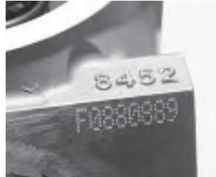
LS7 cylinder heads are identified by the casting number 8452
