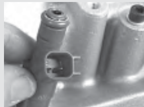
303. Once seated, gently rotate the injector to verify proper O-ring seating.
