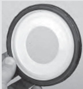
204. The rear crankshaft seal is a one-piece round seal that installs into the rear cover. The inside of the seal rides on the crankshaft's rear flange. However, if the seal (already installed in the rear cover) is simply pushed onto the crank, the seal's front lip will fold rearward, resulting in an oil leak. A white nylon installation tool (seen here inserted into a seal) is needed. This holds the seal's inside lips in proper orientation while the seal is slid onto the crank. This white nylon seal installer is usually supplied with a new replacement seal. If you buy a new rear cover with the seal already installed, you may or may not have this nylon tool. If not, they are available at GM parts counters or any auto parts store.
