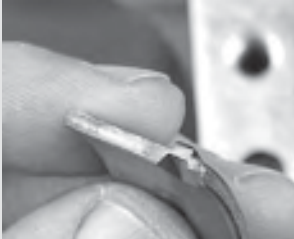
19. Each main (or rod) bearing will feature a tang. This registers into a tang pocket in the block saddle and in the main cap. This locates the bearing during installation in terms of fore/aft location.
