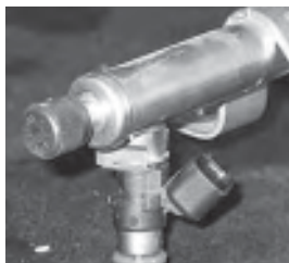
Note that the injectors are secured to the OE fuel rail with metal clips. Set the fuel rail aside until you're ready to install the fuel rail assembly.
