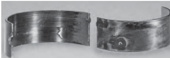
This view shows the damage that results from trapped particles behind the bearing. Note the bearing wear on the face (left). A metal chip that was trapped behind the bearing during assembly distorted the bearing wall inward against the shaft, causing wear through the overlay into the copper-lead base.
