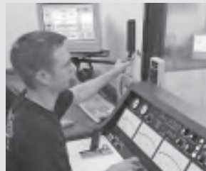
321. Scott controls engine operation at his dyno control center.
