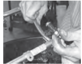
Remove the injectors from the OE fuel rail. Perform this task over a safe area, as fuel will likely run out of the rail.
