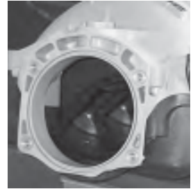
The throttle body port features an O-ring groove for installation of the sealing ring. Note the threaded brass inserts for throttle body mounting.
