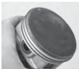
The OE pistons are flat-top. If you plan to run a cam with more than about 0.544" valve lift, you'll need to either notch the OE domes or buy new forged pistons that feature valve relief pockets, to avoid valve-to-piston contact.
