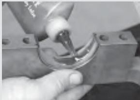
26. With all upper main bearing shells installed into the block saddles, apply a clean lubricant to the entire face of each bearing shell (including the faces of the thrust bearing). You may use clean engine oil, white lithium grease or my favorite, Royal Purple's Max Tuff engine assembly lube.
