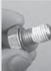
12mm x 1.5 bolt. Install a sealing washer (copper or aluminum crush washer, or an O-ringed Stat-O-Seal) and thread sealant. Unfortunately, you can't buy an OE plug as an individual part (only available with a new GM cylinder head).
