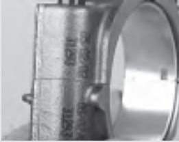
This close-up shows the irregular mating surface between cap and rod, created by the fracture process. This cap has been finger-installed to its rod.
