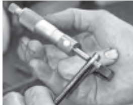
Also measure the valve stem near the top. This non-wear area will provide a reference regarding stem wear on the guide area. The OE valve stem diameter specification is 0.315". Intake valve head diameter should be 2.00" and exhaust valve head diameter should be 1.55".
