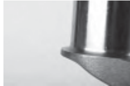
This close-up of a Lunati LS crank shows a nicely rolled fillet on a rod pin. This gentle radiused transition adds strength and eliminates any potential for stress raisers.
