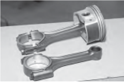
OEM connecting rods in all LS engines (except LS7 and LS9) are powdered metal, (PM) construction. While surprisingly strong for powdered metal, if you plan to build additional ponies, and especially if your plans include nitrous and/or turbo or supercharger boost, trash the OE rods and buy some high quality forged steel rods.
