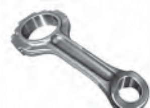
While all other LS engines use powdered metal, cracked cap connecting rods from the factory, the LS7 and LS9 feature forged titanium connecting rods, right from GM.
