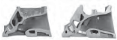
At left is a cross section of an OE LS1 head intake port. At right is a Dart Pro 1. The big differences are the size of the ports, the shape of the ports (note the step in the OE port near the guide boss) and the amount of material Dart added to the top to strengthen the spring seat area and allow for upgraded valvetrain modifications. Courtesy Dart Machinery.
