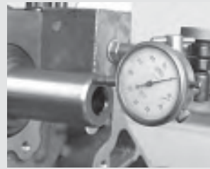
44. Once the main caps have been fully tightened to value, check crankshaft endplay/thrust.
