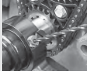
198. This photo shows the drilling fixture mounted to the crank snout for illustration purpose only.
