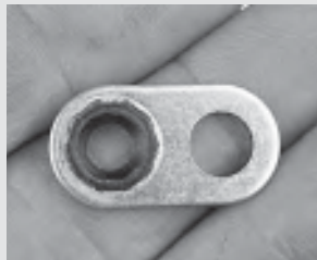
187. In case your block-off fitting is missing its O-ring, GM and aftermarket gasket sets also offers a sealing gasket/plate that sandwiches between the head and block-off.
