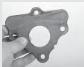
50. The rear of the camshaft retainer plate features a formed-in-place seal. If this seal is damaged, you can carefully apply a thin bead of RTV in the same pattern, or purchase a new retainer plate.
