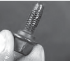
158. Apply thread-locking compound to the lifter bucket 6mm bolts.
