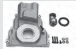
289. Yes, it is possible to run a LS engine not only with a carburetor, but with a distributor (completely eliminating the individual coil packs and timing controller). In fact, this setup was mandated by a Camping World oval track racing series. However, it's expensive. First you need the GM distributor adapter (shown here). This replaces the OE timing cover and accepts a Ford small-block distributor. Since the LS-style camshaft has no drive gear to run a distributor, the adapter kit includes a stubby gear drive that bolts onto the nose of the LS camshaft. Wegner Racing makes this adapter for GM.
