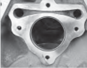
45. The cam bearing tunnel should be cleaned again. While it's nice to precoat the cam bearing faces before installing the cam, if you haven't done this, coating the cam journals will suffice to provide lubricate between the bearings and journals.
