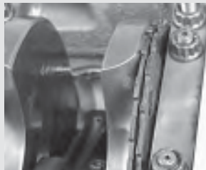
43. Notice the tight location of the reluctor wheel. As long as the wheel doesn't scrape on the No. 5 main cap, you're okay. You'll usually find about 0.100" or more clearance here. Just make sure it isn't bent.
