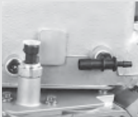
296. The rear of the injection manifold clears the oil pressure tower with ease. A vacuum port at the rear accepts a MAP sensor.
