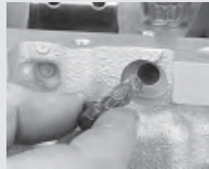
41. Once the 11mm (vertical) main cap fasteners are tightened, apply apply lubricant to both threads and underhead surfaces of the 8mm main cap side bolts.
