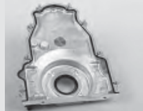
188. Here's a new front cover (purchased from SDPC). An elastomeric sealing bead is pre-installed. If your cover is a used unit, you can use a metal-cored gasket from your gasket kit that features a sealing bead on both sides.
