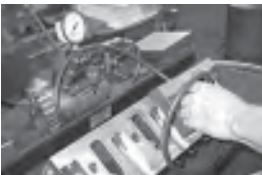
Here the intake valves are checked for sealing. The tester's vacuum gauge will indicate if you have any leaking valve-to-valve seat problems. Any leakdown indicates the need to reface or replace valves and to reface valve seats.
