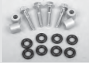
300. If you want to run the taller LS1-style injectors with an LS2-style manifold, you need an adapter kit. Katech's adapter kit is shown here. The fuel rail bracket spacers are 0.500" tall. The bolts are 6mm x 1.0 x 30mm and the O-rings provide the increased outer diameter of the LS2 requirement (to fit the LS2 manifold ports) at about 0.586" O.D.
