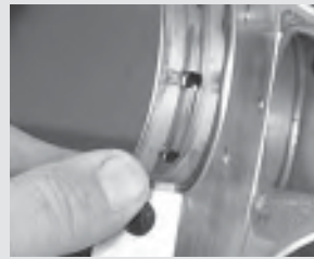
24. Make sure that the bearing edges are reasonably flush with the cap mating surfaces.
