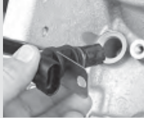
248. Install the crankshaft position sensor with the mounting bracket aimed forward to align with the threaded mounting hole in the block.
