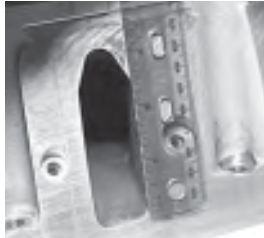
Cathedral ports measure approximately 3.125" in overall height.
