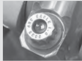
Here we see the dimple on the rod bolt head. These dimples allow the use of a rod bolt stretch gauge to monitor rod bolt stretch during tightening. The gauge features tapered tips that nestle into these dimples.
