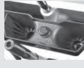
160. A lifter bucket fully installed. Note that the molded shape of the bucket allows installation to the block in only one direction.
