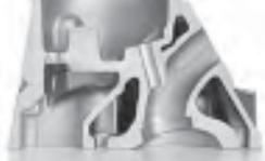
Cutaway view of the LS2 exhaust port for comparison. Courtesy GM.
