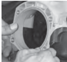
Install a new elastomer sealing ring (supplied in the kit) to the manifold. Do not apply any adhesives. These seals feature a self-gripping design.
