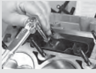
159. Tighten each lifter bucket mounting bolt to a value of 125 in.-lb.
