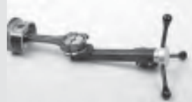
Once a rod cap has been fully tightened to its rod (for checking/measuring purposes, for example), a safe method of separating the cap is with the use of a dedicated rod cap splitter tool. This draws the cap from the rod without the need to hold the rod upside down and bang on the loosened rod bolts.
