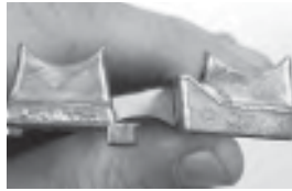
This end-view of the two rocker rails shows the early LS1, LS6, LS2 rail at the left and the later LS3, LS9, L92 rail at right.
