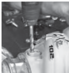
Using a 15/32" drill, fully drill through the MAP sensor port location.
