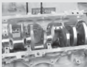
27. Carefully lay the crankshaft into position. Use extreme care to prevent nicking crank journals and to prevent damaging the upper main bearings. Once the crankshaft is lowered onto the block's main saddles, do not rotate the crank.
