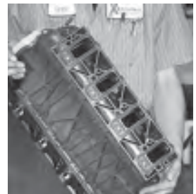
The underside of the FAST manifold features a network of strengthening ribs, the result of extensive research and development.
