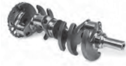
For a drastic weight/mass reduction, superlight crankshafts for high rpm racing applications can feature severely scalloped counterweights. This Callies Magnum XL is a good example of a no-holds-barred racing crank that features reduced mass while maintaining race-level durability. Courtesy Callies.
