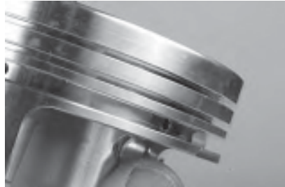
Today's thinner piston rings also help to accommodate shorter ring land areas in short-CD pistons. For LS applications, the 1.5mm, 1.5mm, 3mm top-second/oil layout is typical.
