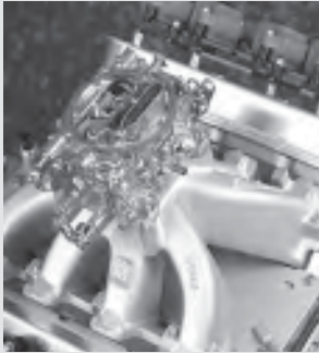
284. Even if you elect to run a carburetor, you still need the coil packs, and you'll need a timing controller to fire the coils (unless you decide to run a distributor, which we'll discuss shortly).
