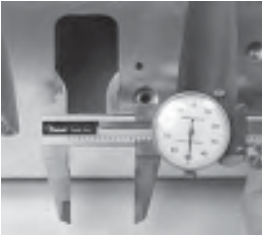
The LS3, LS9 and L92 intake ports measure about 1.250" wide.
