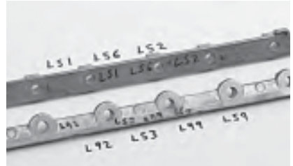
This underside view of the early (seen at top in this photo) and later rails shows a clear shape difference. Note the later rail (seen at bottom in photo) bolt holes are slightly offset and the hole bosses protrude outward on one side.
