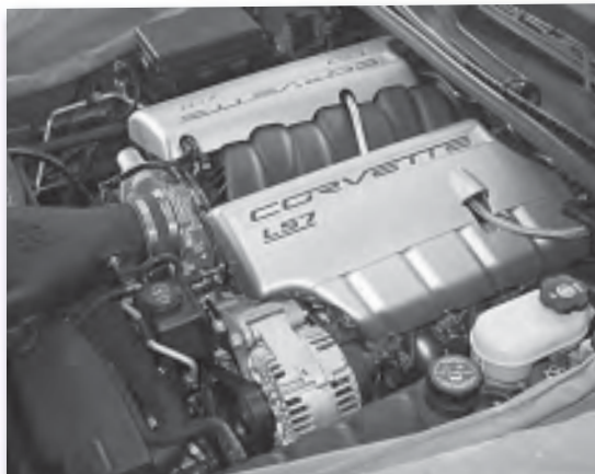
Although this chapter details an intake manifold swap on a Z06 Corvette equipped with the LS7 engine, the procedures are similar for other LS models.
