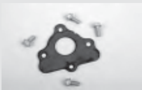
49. The camshaft is secured in the block via a camshaft retainer plate. This plate is secured to the block with four screws. The nose of the camshaft is stepped. The smaller diameter nose section will pass through the retainer plate center hole. Be sure to apply lube to the cam nose (the step shoulder) before installing the retainer plate. Also, apply thread locking compound to all four screws. Tighten the four retainer plate screws to a value of 18 ft-lb.
