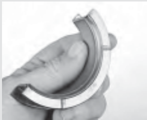
22. The two-groove side of this Clevite thrust bearing must face toward the front of the block.
