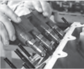
155. With all lifters fully lubed with oil and installed into their respective lifter buckets, gently install the lifter bucket, aligning the lifters to the lifter bores.
