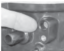
The rear MAP sensor location is at the rear-right area of the manifold. Depending on your application (the stock location of your MAP sensor), you'll need to drill the sensor mounting hole.
