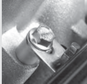
306. Closeup of a fuel rail bracket with 30mm bolt and 0.500" spacer.
