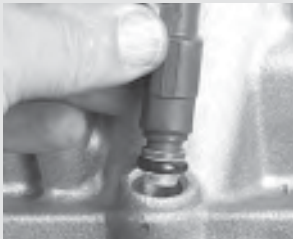
302. Be sure to lubricate the injector O-rings (top and bottom) with lithium lube before installing, to prevent O-ring damage.
