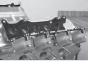
281. Here the coil packs are installed to the top plate and hinged away from the base plate.
