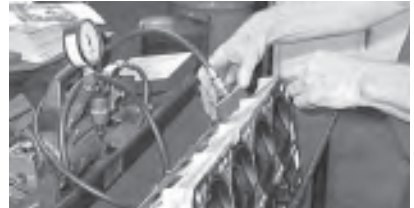
With valve springs removed, vacuum test each valve location. Here the exhaust valves are checked for sealing.
