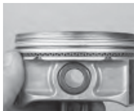
This side view of an OE LS piston and ring package shows the 1.5mm top ring, 1.5mm second ring and 3mm oil ring package. When building a stroker engine, you may need a piston that features a shorter compress distance (centerline of the wrist pin to the dome) to avoid raising the piston too far above the block deck.
