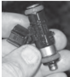
Inspect the fuel injector's O-rings (upper and lower). It's always a good idea to replace all O-rings whenever servicing injectors.
