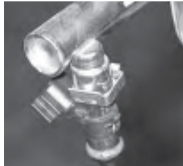
If you plan to use new billet fuel rails, remove the injectors from the stock fuel rail. Remove the retaining slip that secures the injector.
