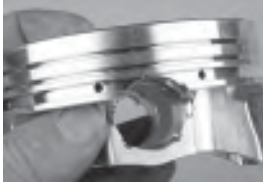
A piston's compression distance (CD) refers to the distance from the centerline of the wrist pin bore to the flat surface of the dome.
