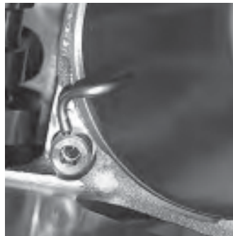
Piston oil squirters were added to the LS9 block to reduce under-piston temperature. The use of oil squirters is a common approach in several engine designs, including the Honda B18C1 engine block to name but one example. Courtesy GM.
