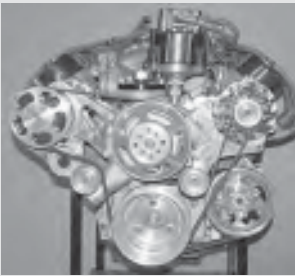
293. You'll also need a completely new pulley setup to align with the new location of the water pump pulley. (Courtesy Wegner).
