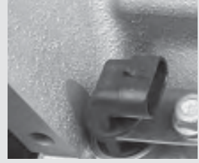
249. The crankshaft position sensor is secured with an 8mm x 1.25 bolt. Use a short bolt, about 10-15mm long, since this blind hole is only about 19mm deep at the most.
