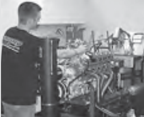
317. The cooling tower (black vertical tube in foreground) pressure-routes water through the engine's cooling passages, so no finned radiator is needed for dyno operation.
