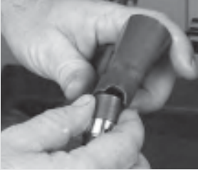
152. Lube the lifter with oil and insert into the bucket.
