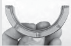
21. The LS engine features the thrust bearing in the center (No. 3) main bearing location, unlike early Chevy engines. The Clevite main thrust bearing features three grooves on one thrust face and two grooves on the opposite thrust face. The three-groove side must face toward the rear of the block.
