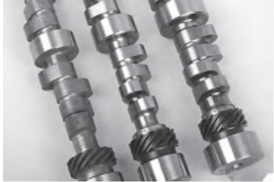
Note that both the 4/7 swap cam (center) and the LS cam (right) both feature the second and fourth lobes from the front in an opposed position as compared to the stock firing order cam.
