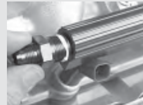
307. The front of each aluminum fuel rail accepts a 3/8" NPT to -6 AN male/male fitting. This allows connection of the -6 crossover hose that plumbs the two fuel rails together. Note the injector connector aiming outboard for wiring harness connection.
