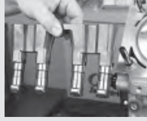
154. With four lifters fully installed into a lifter bucket, the group of four lifters can be installed into the block.
