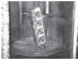
Once the cylinder heads have been completely disassembled, they should be cleaned in a hot tank or heated pressure-washer to remove oil and contaminants.
