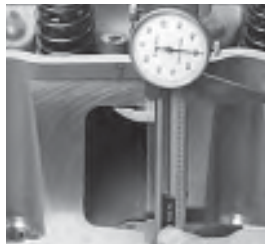
The LS3, LS9 and L92 intake ports measure about 2.550" high.
