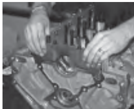
With main studs in place, the main caps are re-installed.
