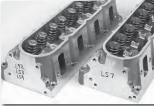
The later Gen IV LS cylinder heads basically include two different heads, one for the LS3, LS9 and L92 (left) and one for the LS7.
