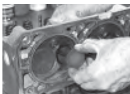
Once the leakdown test has been completed, remove the intake and exhaust valves.
