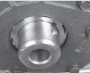
203. While you can remove the new key pin and reinstall it after the oil pump is installed, locating the new pin in line with the existing crank gear key allows you to service the oil pump without the need to mess around with the new pin.
