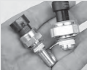
250. Coolant temperature sensor (left) and oil pressure sensor.
