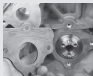
51. Make sure that the mating surfaces (block and rear of retainer plate) are clean and dry.
