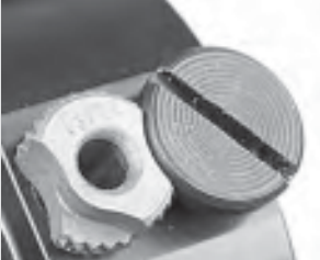
197. The drilling mandrel features a drill guide that is secured with an adjacent screw head.
