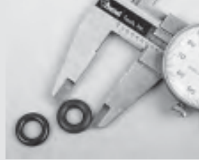
301. An intake manifold that is designed for LS2 injectors features a larger diameter injector port as compared to an LS1 manifold, so if you plan to run LS1 style injectors in an LS2 manifold, you need the larger-diameter 0.586" O-rings.
