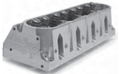
Edelbrock rpm Xtreme LS-series as-cast cylinder head features CNC porting in chambers, intake entry, exhaust exit and intake/exhaust bowls. Courtesy Edelbrock.
