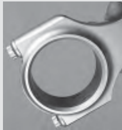
Even when using the best aftermarket rods, always check big- and small-end bore diameters, just to be sure.
