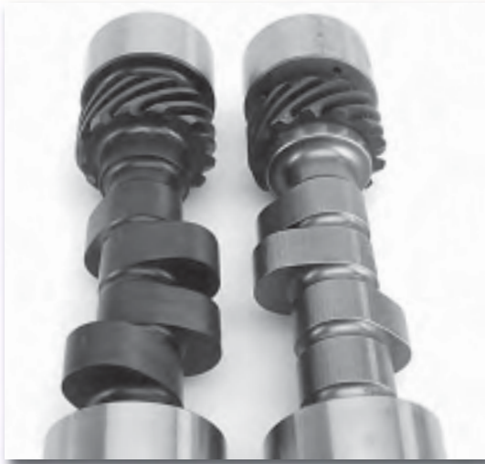
The cam on the left is a standard firing order big-block Chevy. The cam on the right is a 4/7 swap cam. Notice that the second and fourth lobes from the rear on the 4/7 are opposed vs. the standard cam. This is an easy way to identify a 4/7 swap cam. Courtesy Comp Cams.
