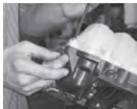
Before drilling for the MAP sensor, disassemble the upper and lower manifold sections to prevent plastic debris from being trapped. Using a hex wrench, remove the socket head cap screws that secure the two halves together. The nuts are located inside hexagonal passages in the lower section.
