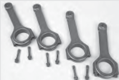
Aftermarket performance connecting rods are available in both I-beam (similar in shape to the OE rod beam) and H-beam (seen here). Generically speaking, I-beam type rods are OK for anything up to about 400 hp. Beyond that, H-beam rods are recommended due to their greater design strength.
