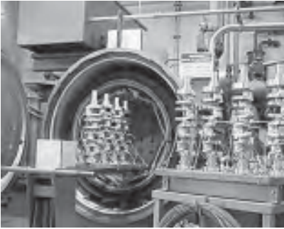
Surface hardening such as ion nitriding is done by exposing the cranks to an ammonia/nitrogen mix, where nitrogen reacts with the surface, creating a hardened surface. Hardening depth is controlled and dictated by the specific manufacturer. Courtesy Bryant.
