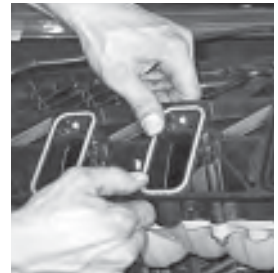
Install new intake port seals to the manifold (also supplied in the FAST kit).
