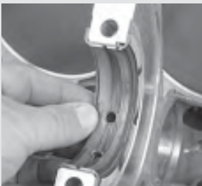
25. The thrust bearing is installed at the No. 3 main bearing location. Again, make sure that the 3-groove side of the thrust face aims toward the rear of the block.
