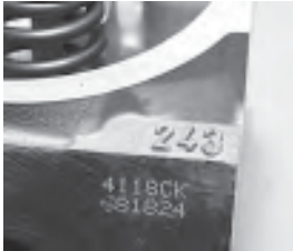
Both LS6 and LS2 cylinder heads feature a casting number of 243.
