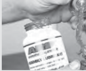
38. If using main cap studs, apply a bit of lube to both sides of the washers (or nuts flange, depending on fastener style) and to the threads and underside of the nuts. Here I apply ARP's moly lube.
