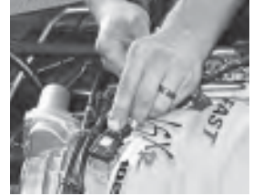
Reconnect coolant crossovers and all vacuum lines. Reconnect the MAP sensor harness.
