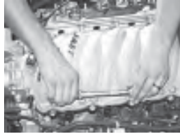
Tighten the manifold mounting screws in the proper sequence initially to 45 in-lbs, then to a final value of 70-89 in-lbs. It's important to follow the tightening sequence to obtain even load distribution.
