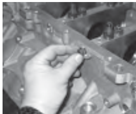
If you're using main cap primary bolts, first coat the bolt threads and underside of the heads with oil or moly. If using studs, apply oil or moly to the exposed stud threads, nut threads and underside of the nuts. Once the primary 10mm main cap fasteners are torqued to value, coat the threads and the underside of the bolt heads of the side cap bolts with oil or moly.
