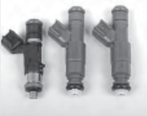
299. This photo illustrates relative height differences. At the far left is an LS2 injector at 2.575" tall and two LS1-style injectors at 2.917" tall. O-ring diameters vary as well, depending on the intended manifold fit.
