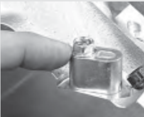
186. Here a block-off is installed on the rear of a cylinder head. The rears are always blocked off.
