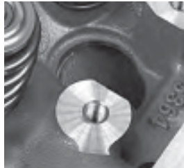
This close-up shows the flat-machined bosses. A one-piece cast aluminum rail mounts atop these bosses, with the rails featuring the radiused rocker locations.
