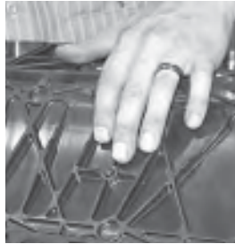
The underside of the manifold requires the installation of three rubber bump-stops. These are self-adhesive. Here Brian's middle finger points to the center bumper.
