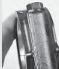
As you begin to tighten the rod bolts, the once-noticeable separation crack begins to disappear. Once fully tightened, you cannot see the mating line at all. Powder metal construction with cracked caps are nothing new and are not unique to LS rods. This OE-only design has been around for many years.
