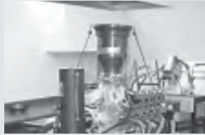
318. A huge air inlet ducts air to the air inlet stack that's fastened to the carb. With ignition connected and water temperature, oil pressure, ambient air temperature, fuel pressure, exhaust gas temperature and barometric pressure monitored, she's ready to fire.
