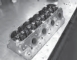
Once the OE heads have been partially disassembled and vacuum tested, they'll be cleaned in a hot tank or pressure washer.
