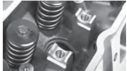
The LS7 heads do not require separate rocker rails, since the head casting features machined radiused pockets to directly accept the rockers. Many aftermarket performance LS-style cylinder heads also feature these rocker pedestals, eliminating the need for rocker rails.
