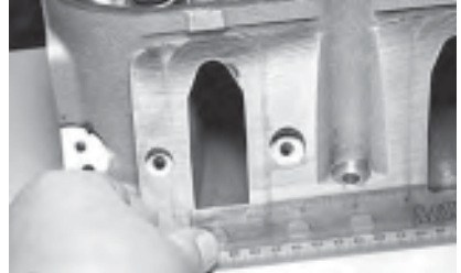
Cathedral ports measure approximately 1" in width.
