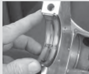
23. Install the bearing shell with the registration tang mated into the saddle's tang cutout, and press both ends of the bearing shell into the saddle with your fingers.
