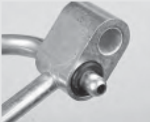
183. The front-mounted crossover pipe connects the two heads together and allows the heads to share a common steam evacuation path to accommodate the OE vehicle system. The tube that enters the steam hole is fitted with a sealing O-ring.
