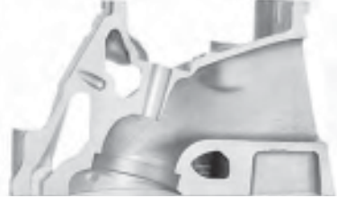
Cutaway view of the LS3/LS9 intake port. Courtesy GM.
