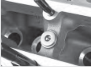
156. Some performance roller lifters may be taller than the OE lifter. If so, the lifter maker will provide spacer washers to move the lifter buckets up slightly. If so, the spacer must be placed on the block surface, centered with the lifter bucket mounting bolt hole before the lifter bucket is installed. If these spacers are needed, apply a dab of assembly lube onto the bottom of the spacer first to prevent the spacer from sliding off before the lifter bucket bolt is installed.
