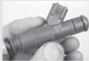
298. The injectors I picked for our injected version of Project LS2 are Bosch P/N 0280 156 127. These are the taller LS1 style, measuring about 2.91" tall.
