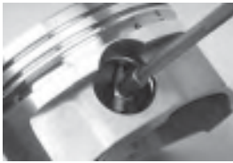
Here we use a bore gauge, adjusting it to duplicate the piston's pin bore. The snap/telescopic bore gauge is then carefully measured with a micrometer.
