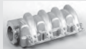
295. There are a number of multi-port electronic fuel injection systems currently available for the LS platform (Edelbrock, FAST, etc.). As an example, here's a injection manifold from Professional Products (their Power Plus Typhoon model P/N 52063). It's a cast aluminum manifold that accepts a 90mm throttle body. Blank bosses are provided if you elect to install nitrous injection.
