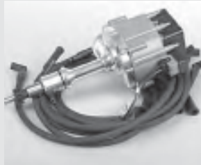
291. This distributor is earmarked for a Ford, but features the convenience of a GM type HEI integrated coil. Yes, it works with the LS, as the adapter kit's cam drive gear and adapter housing distributor depth was designed with the Ford unit in mind.
