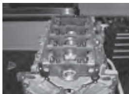
If you're using main cap primary bolts, first coat the bolt threads and underside of the heads with oil or moly. If using studs, apply oil or moly to the exposed stud threads, nut threads and underside of the nuts. Once the primary 10mm main cap fasteners are torqued to value, coat the threads and the underside of the bolt heads of the side cap bolts with oil or moly.
