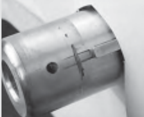
201. The new key pin hole must be in line with the existing crank gear key, to allow installation of the oil pump's keyway, which will pass over this pin and engage on the crank gear's key. This will also make it easier to remove the crank gear at a later date. Here you see marks that were made before drilling to achieve this alignment.
