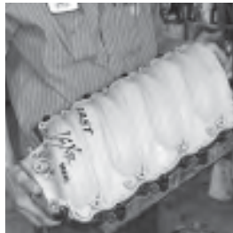
The FAST manifold is a bit taller than the stock unit, requiring either the use of injector spacers along with the stock fuel rail assembly, or the use of FAST's billet fuel rails.
