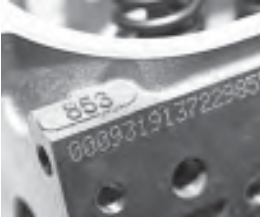
LS cylinder heads feature a handy three-digit casting identification number. Shown here is an LS1 head with casting number 853. LS2 cylinder heads are marked with number 243.
