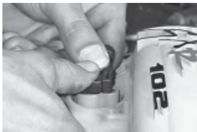
Gently push the MAP sensor probe into the drilled hole (make sure that the sensor's silicone seal is not damaged). Secure the MAP sensor using the screw provided in the FAST kit. Tighten gently. Do not tighten to more than 19 in-lbs.
