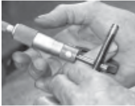
Use a micrometer to measure each valve stem. Measure the lower area of the stem that rides through the valve guide and record the diameter.
