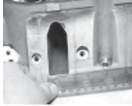
The LS1, LS6, LS2 type of head features cathedral shaped intake ports (tall with tapered tops) and are about 1" wide.
