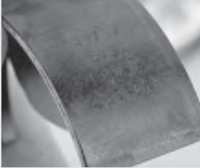
114. This bearing is marked "LOWER" and must be installed to the rod cap.
