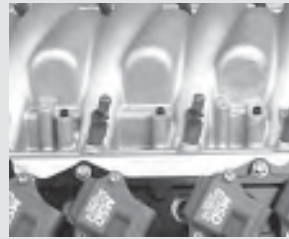
304. All eight injectors installed in the manifold and ready for fuel rails. Be sure to rotate the injectors to orient the connectors outward to provide wiring harness access.
