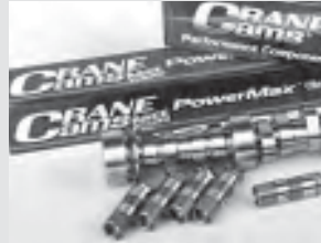
46. A wide variety of camshaft profiles are available for the LS engine family. I chose a custom grind from Crane. All LS cams are the roller type (usually made from steel billet). It's generally best to use the same make roller lifters.
