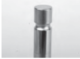
Applying a hard coating such as TiN to the stem tip and lock groove protects the titanium material from galling damage from a lash cap and retainer locks.
