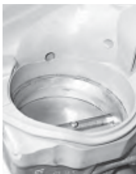
This inside view shows the hole that Brian drilled. Dress the hole edges to remove any burrs.
