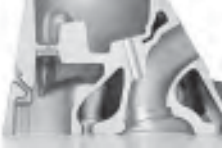
Cutaway view of the LS3/LS9 exhaust port. Although subtle, the roof of the port on the LS3/LS9 exhaust path rises a bit for a smoother exit path. Courtesy GM.
