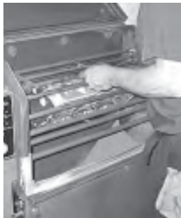
A nice way to final-clean the head surfaces is to tumble-blast the head in an enclosed blasting cabinet using a soft cleaning media such as walnut shell particles.
