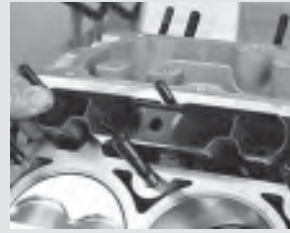
157. With the group of four lifters entering their respective lifter bores, allow the bucket to rest onto the block mounting surface.
