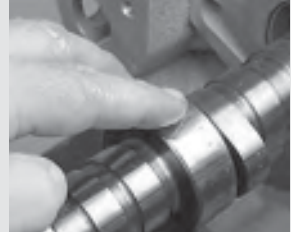
47. Apply a generous amount of lubricant to the camshaft journals and lobes. Start by lubricating only the rear two journals and the rearmost lobes. As the cam is carefully inserted into the first two bearing locations, you can then continue to apply lube. This makes the cam easier to maneuver. Use extreme caution when installing any camshaft to avoid nicking or gouging the cam bearings. The camshaft must be kept perfectly aligned to the cam bores. If you feel any resistance, do not force it. Gently wiggle the cam to engage the journals into the bearings as you proceed.
