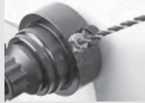
199. If the damper key pin drilling procedure will be done with the crankshaft in the block (obviously not preferred), the front of the engine block must be shielded to prevent particles from contaminating the engine. With the installer mandrel in place and secured with a damper bolt, a 0.1690" hole is drilled into the crank snout, all the way through to the snout centerbore.
