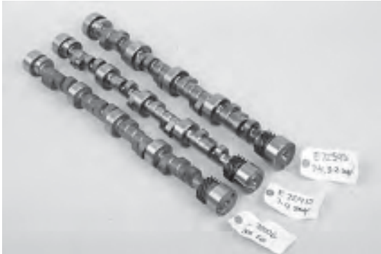
Shown here are three Erson big-block Chevy cams (from left to right): a standard firing order, a 4/7 swap and an LS firing order cam.
