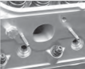
253. This photo shows the plugged water port on the right side cylinder head, immediately behind the No. 8 cylinder exhaust port. This isn't a hillbilly fix...it works just fine.
