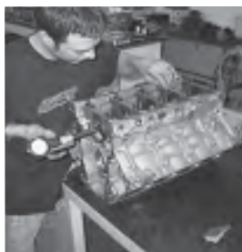
Scott Gressman of Gressman Powersports finalizes his check of main bore dimensions.
