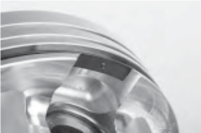
This view shows the small bump (male dimple) on the underside of the oil ring support rail. This provides a positive stop in case the support rail begins to rotate, preventing the support rail gap from entering the void.
