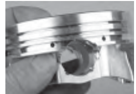
Due to the short CD on this piston (1.115"), the pin bore is positioned high enough that it intersects the oil ring groove. In this situation, a special oil ring support rail is needed (the piston maker widens the oil ring groove to accommodate the addition of the support rail).
