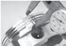
Here we measure from the top of the wrist pin bore to the piston dome. Add to this the radius of the pin bore to determine the piston's compression distance.
