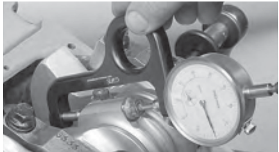
You have a choice of two methods for rod bolt tightening (when using performance aftermarket rods and rod bolts): torque or stretch. Rod (and bolt) makers will provide both specs. The stretch method offers a more accurate way to monitor and achieve desired bolt clamping load, since the torque factor is eliminated (by monitoring only tightening torque, the variable of thread and bolt underhead friction can result in slight inconsistent bolt tightening. Each engine builder has his own preference (torque or stretch). Shown here is a Gearhead Tools stretch gauge that features a handy finger hole for holding the gauge.
