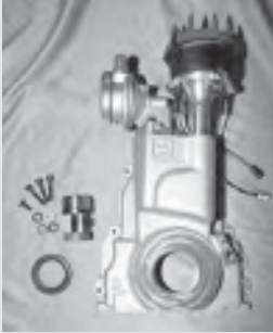
290. Here's a sample adapter housing, camshaft gear drive and distributor. Courtesy Wegner.
