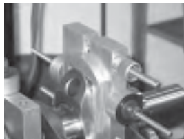
Bobweights need to be centered (fore/aft) on each rod pin. Here Scott Gressman temporarily installed a custom-made aluminum spacer which allows him to quickly center the bobweight without taking the time to measure.
