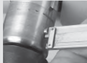
202. One of the kit's 3/16" pins is tapped into the drilled hole and is set at an exposed height of 0.093". Here we check the height with the depth-gauge of a caliper.
