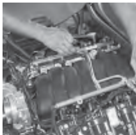
With the fuel injector harnesses disconnected from all eight injectors, remove the OE fuel rail assembly, gently wiggling and pulling to remove the fuel injectors from their intake manifold ports.
