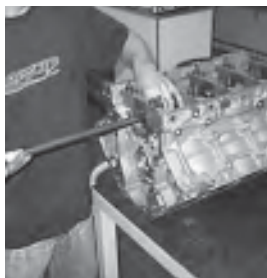
With main caps fully installed, main bores are checked individually for size/roundness consistency. This check reveals need for resizing corrections at each main bore location.
