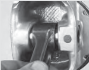
As noted earlier, the OE connecting rod small ends are interference-fit to the piston wrist pins. The pin floats inside the piston's pin bore, but remains locked to the connecting rod. Performance aftermarket rods and pistons offer full-float design, where both the piston and the rod pivot (float) with an oil clearance between both piston pin bore and rod pin bore.
