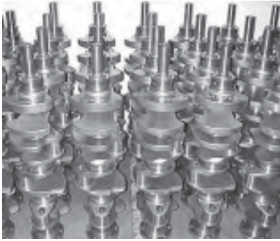
Finished forged cranks ready for inspection. Courtesy Bryant.
