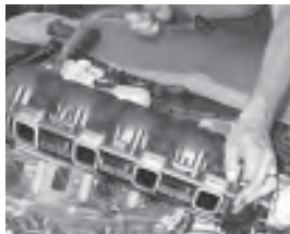
With all intake manifold bolts removed, and verifying that the rear vacuum hose connections have been disconnected (and the MAP sensor disconnected, if your application features a rear-mounted MAP), carefully remove the intake manifold. Make sure that no debris falls into the exposed cylinder head intake ports.
