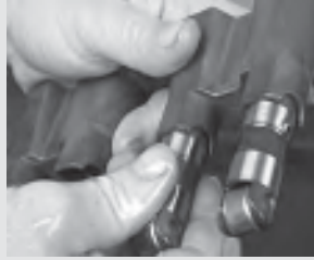
153. Push the lifter full up into the bucket. It will gently "click" in the up position.
