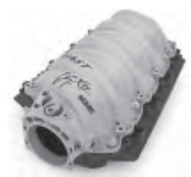
The FAST LSX R manifold that we're installing in this example features a 102mm throttle body port. The precision molded composite manifold is designed as a 2-piece assembly.
