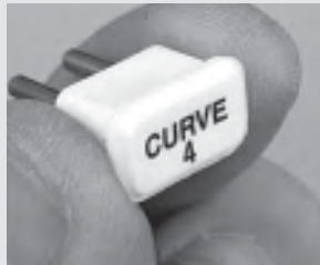
288. Each timing curve plug-in module is labeled. MSD's instructions provide the details of each module's characteristics. However, you can create your own custom curves by using the software CD provided in the kit. It's not complicated at all. Plug a laptop or desktop PC into the timing control unit and map your own timing curve. We did this during my LS2's dyno session, and it was easier than I thought it would be.
