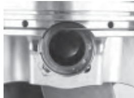
This side view shows the oil ring support rail in position. This is installed prior to installing the oil ring package.
