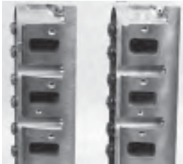
Both the LS3, LS9 and L92 head (left) and the LS7 head (right) feature rectangular intake ports, unlike the cathedral ports used on Gen III LS1, LS6 and LS2 heads.
