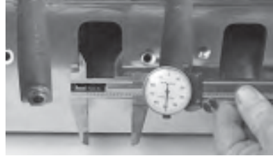
The LS7 intake ports measure 1.350" wide.
