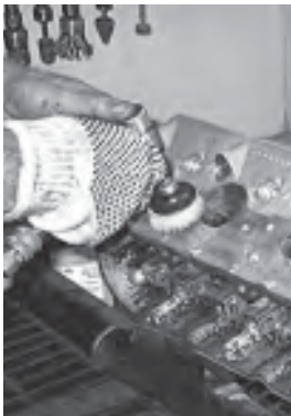
A Rodex cleaning brush can be used to quickly final-clean the intake and exhaust decks. Don't dwell on isolated areas to avoid creating uneven surfaces.
