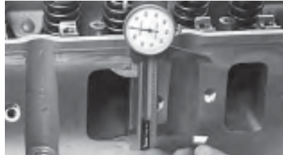
The LS7 intake ports measure 2.40" high.
